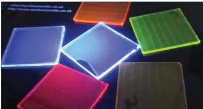
Fig. 19 Intensely fluorescing films of CSAR 62 on glass.
