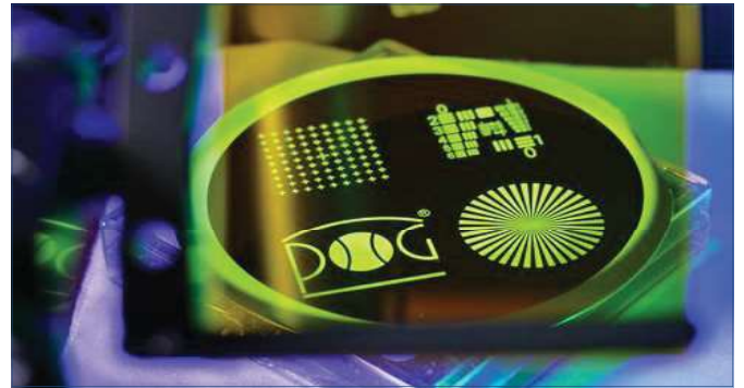
Fig. 21 Yellow fluorescent PMMA-based resist architectures
